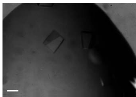
Figure 1 Crystals of NusA as grown by the hanging-drop method. The average dimensions of these crystals are 150 × 100 × 80 µm. The scale bar is 100 µm in length.
